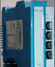
The 2C50 Ethernet 10 BASE-T 4-Port Hub Module performs repeater functions to and from its four ports. Preamble regeneration, data collision detection and segmentation are built in functions of the Ethernet hub design.
